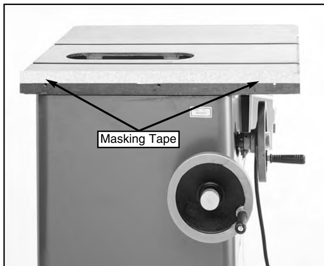
Figure 7. Using tape to shim for wing alignment.
